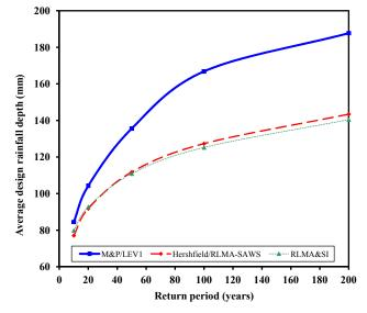
**Figure 7**Average design rainfall depth:  $6 < T_c \le 24 \text{ h}$
