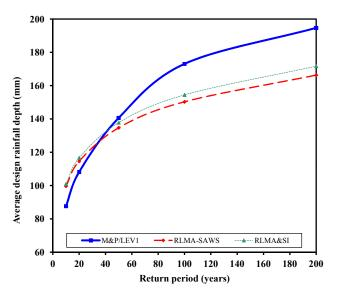
**Figure 8**Average design rainfall depth:  $24 < T_c \le 168 \text{ h}$
