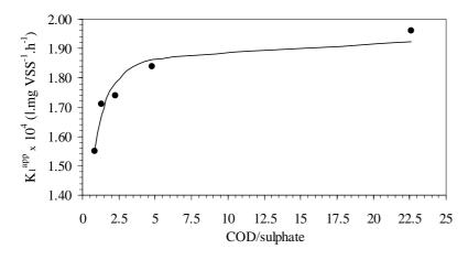
Figure 2 Apparent first-order kinetic parameters as a function of COD to sulphate ratio. Experimental values (•) and adjusted expression ( –).
