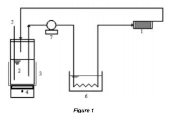
Experimental apparatus to estimate kinetic parameters. (1) Differential reactor; (2) Agitated tank; (3) Ice batch; (4) Magnetic stirrer; (5) Sampler; (6) Heat exchange; (7) Peristaltic pump.
