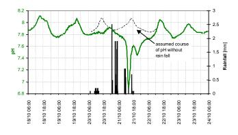
**Figure 7** Response of the pH-value in the Koekemoerspruit to an acid rain event (observation period 18 -24 Oct 1999)
