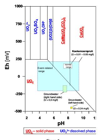
**Figure 9** A pH-Eh-stability diagram for 1 μM U in dolomitic water in comparison with the range of pH and Eh values observed in stream and groundwater at the study site
