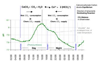
**Figure 4** Processes controlling diurnal pH oscillations in the Koekemoerspruit (illustration based on an example of the pH-cycle observed on 8<sup>th</sup> October 1999)
