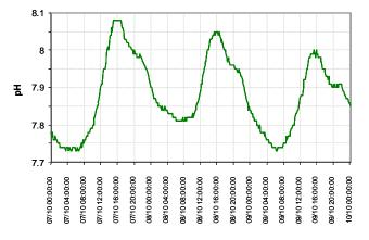
Figure 2 Diurnal fluctuations of the pH in the Koekemoerspruit (observation period: 07-10 October1999)
