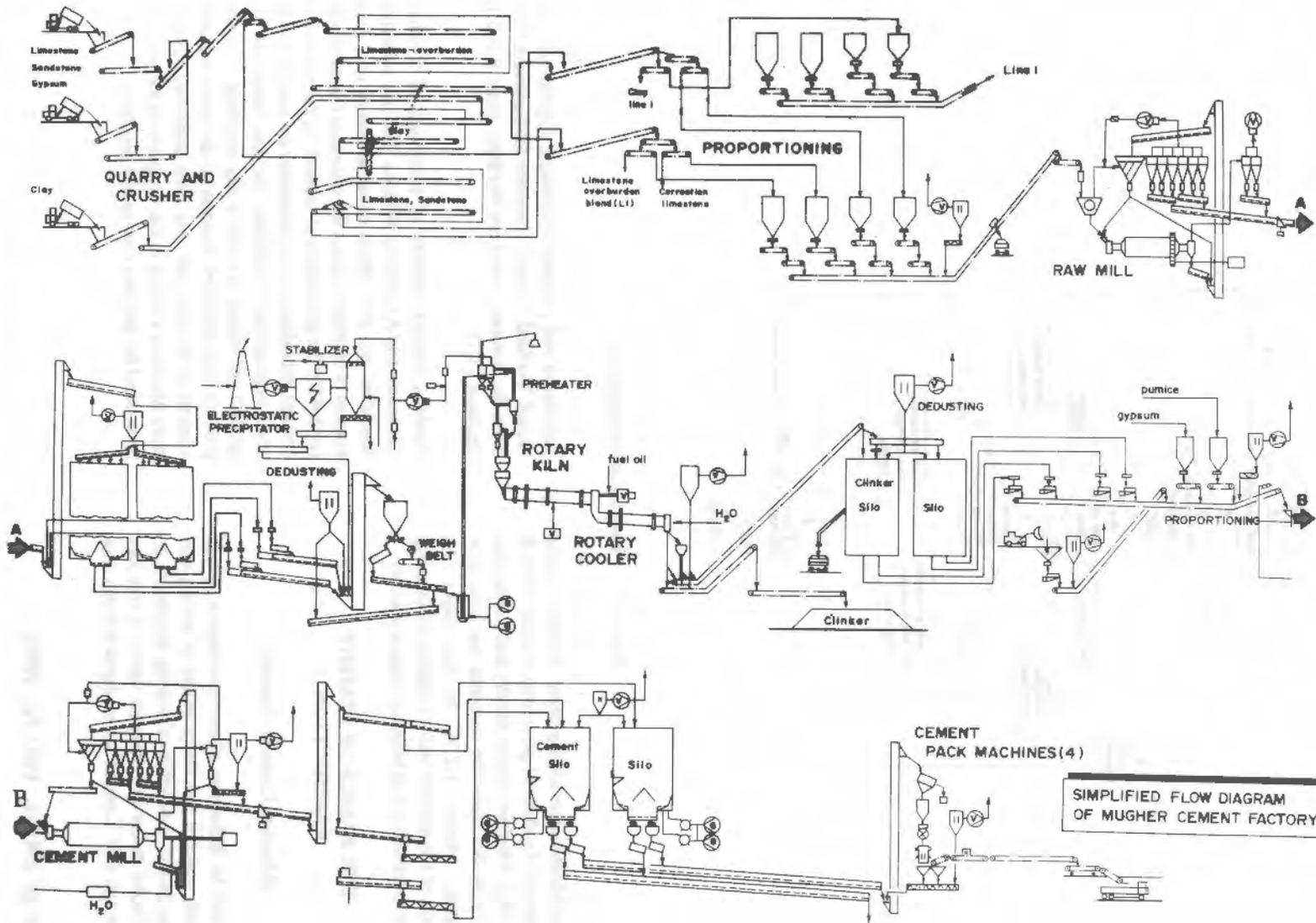
Figure 5 Simplified Flow Diagram of Mughet Cement Factory
