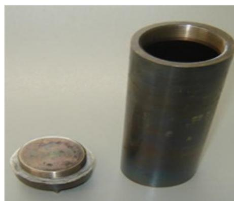
Figure 2. Titanium extractor.
