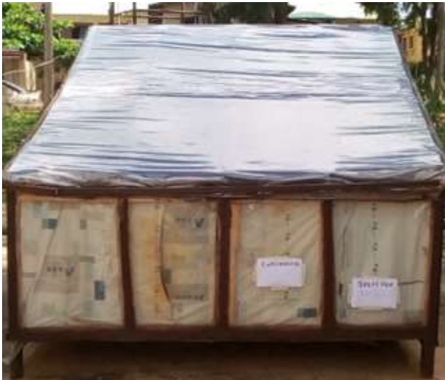
Figure 1. The greenhouse-type solar kiln used for drying Khaya ivorensis timber.
