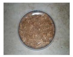
Figure 7. Sisal bole chips dried at 150 °C.
