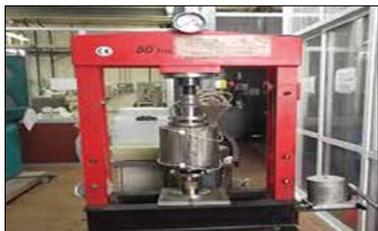
Figure 1a: Hydraulic press machine
