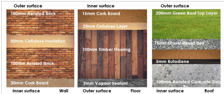
Figure 4: Second optimised model: Wall, floor, and roof composition
