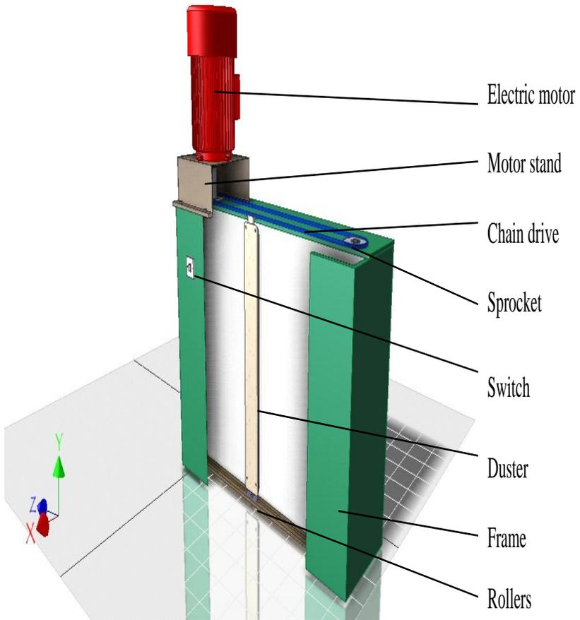
Figure 1: Isometric view of automated whiteboard cleaner
