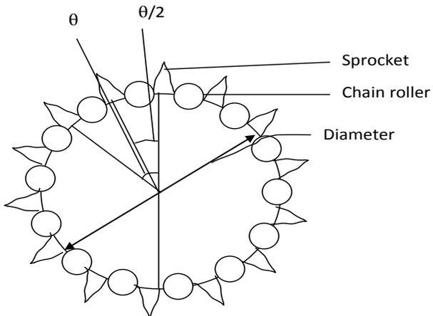
Figure 4: Type of sprocket used in chain drive
