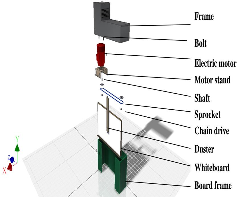
Figure 2: Exploded view of automated whiteboard cleaner
