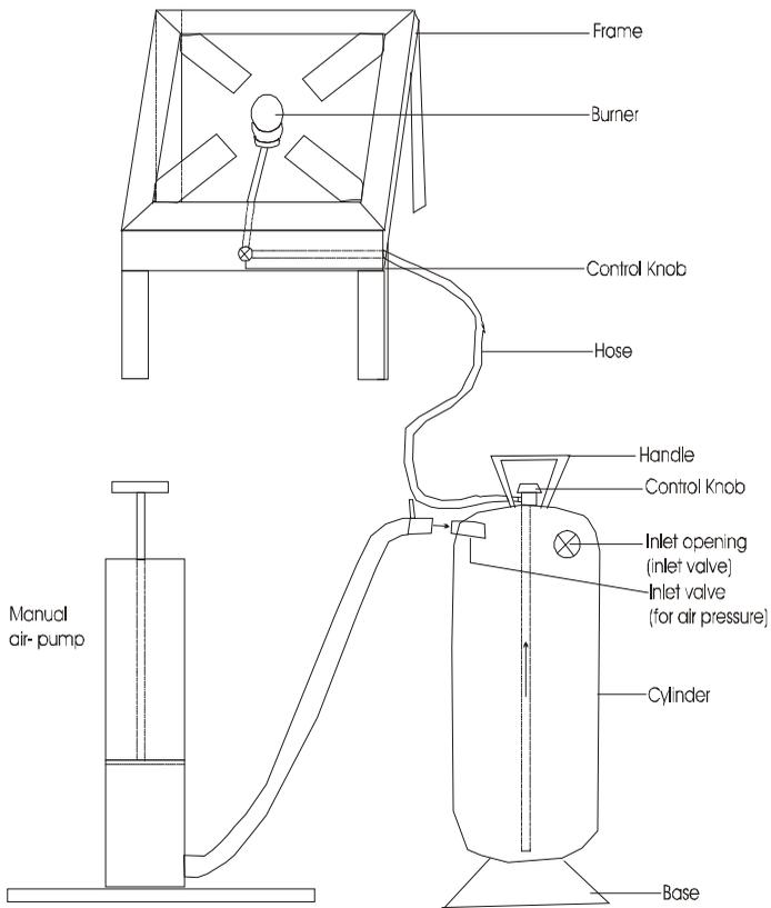
Fig. 6 Assembly of Kerosene pressure - cooker
