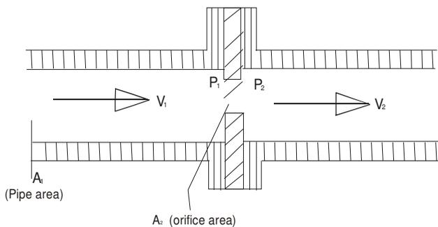
Fig. 4. Flow through an orifice
