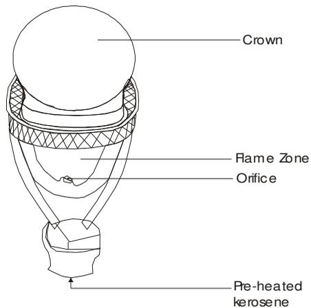
Fig. 2 Pressure burner (Atomizer)
