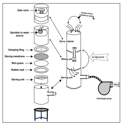
Figure 2: The fluid and air flow in suction sieving
