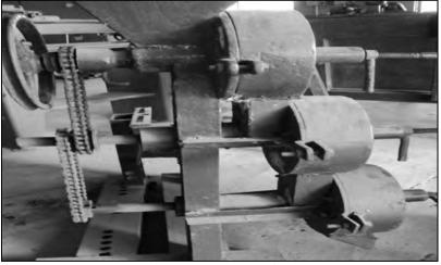
Figure 4: The Multi-stage Grinder
