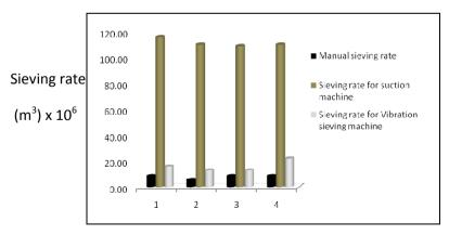
Figure 5 Sieving Rates for Manual and Mechanical processes
