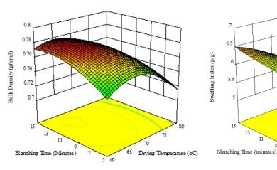
Fig. 2. Variation of bulk density with blanching time and drying temperature
