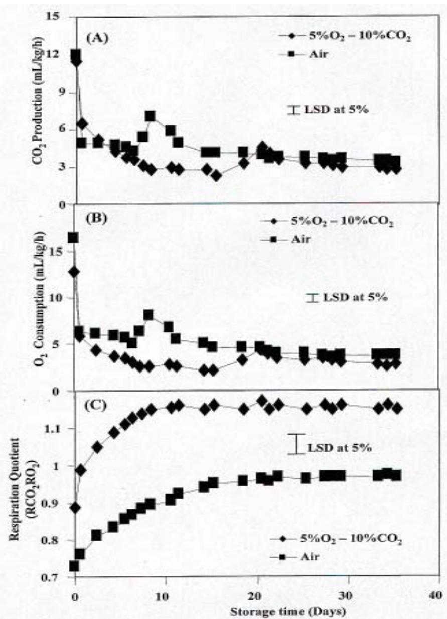
**Figure 4 :** Respiration rate and respiration quotient (RQ) of tomatoes stored in controlled atmosphere (5 % O<sub>2</sub> - 10 % CO<sub>2</sub>) and in air conditions at 13° C.
