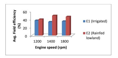
Figure 4: Effect of engine speed on field efficiency at different ecologies
