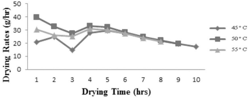
Figure 3: The effects of Drying Temperature and Time on Drying Rate for 300g *Iru Woro*
