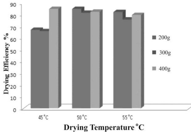
Figure 8: The effects of Drying Temperature on the Drying Efficiency of the Dryer for *Iru Woro*
