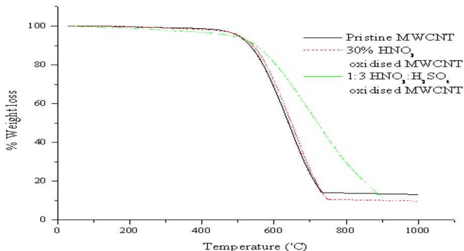
**Figure 4: Thermal stability of pristine, 30% HNO<sub>3</sub> and 1:3 HNO<sub>3</sub>:H<sub>2</sub>SO<sub>4</sub> oxidised MWCNTs**
