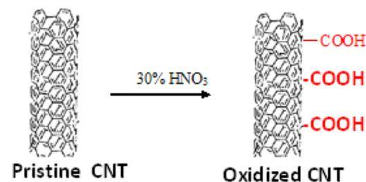
**Figure 1: Oxidation of pristine MWCNT to create MWCNT-COOH**
