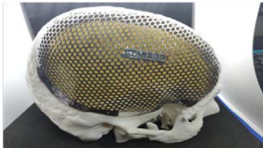
Figure 9: SLM Printed Ti implant
