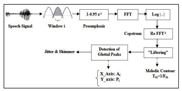
Figure 1: Block diagram of the calculation of Jitter and Shimmer
