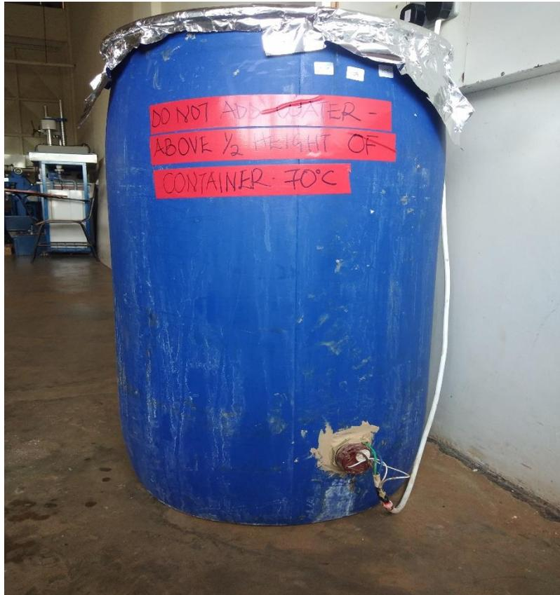
*Figure 2: Plastic drum used as a curing tank.*
