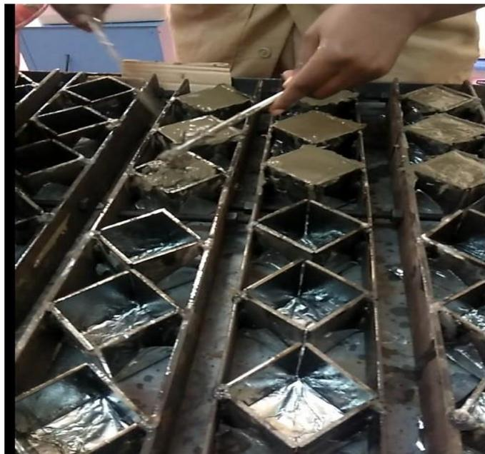
*Figure 1: Image of moulds that were used to prepare the specimen*
