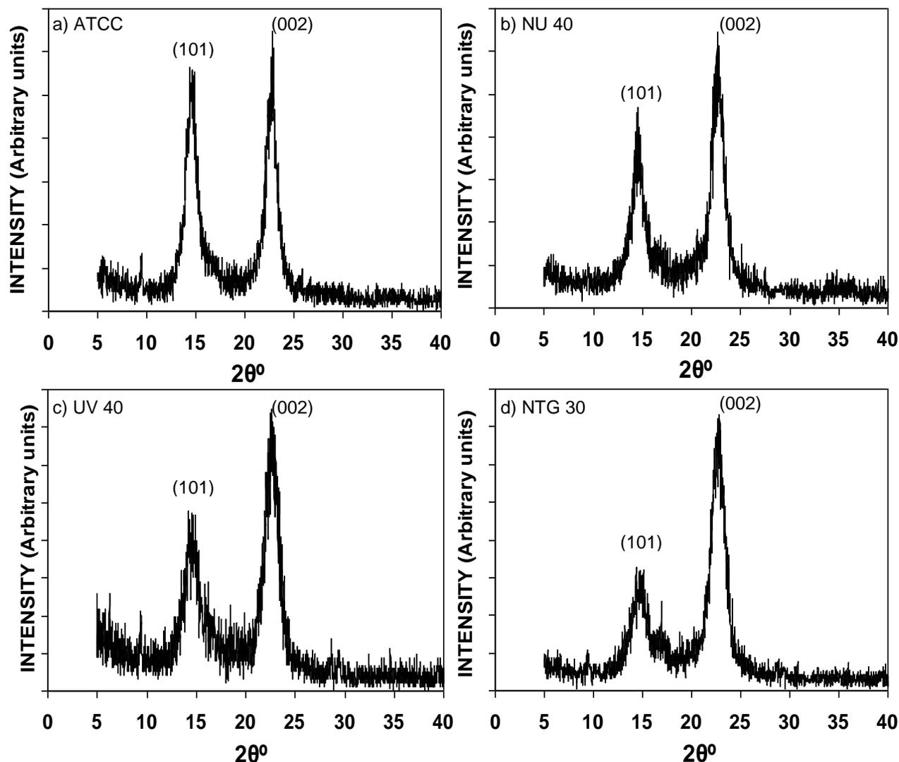
**Figure 3.** X-ray diffractograms of cellulose pellicles produced by (a) reference strain *A. xylinum* ATCC 10245, (b) *Acetobacter* isolate NU4, (c) mutant NU4-UV40-07 and (d) mutant NU4-NTG30-51.
