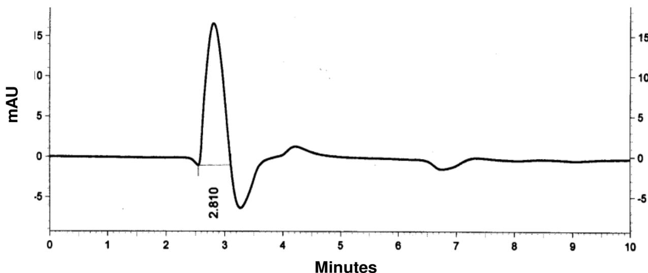
**Figure 2.** HPLC chromatogram of authentic Cyclosporin 'A' purchase from Fluka, Japan. The chromatogram extracted at 215 nm is showing Cyclosporin 'A' peak at 2.8.
