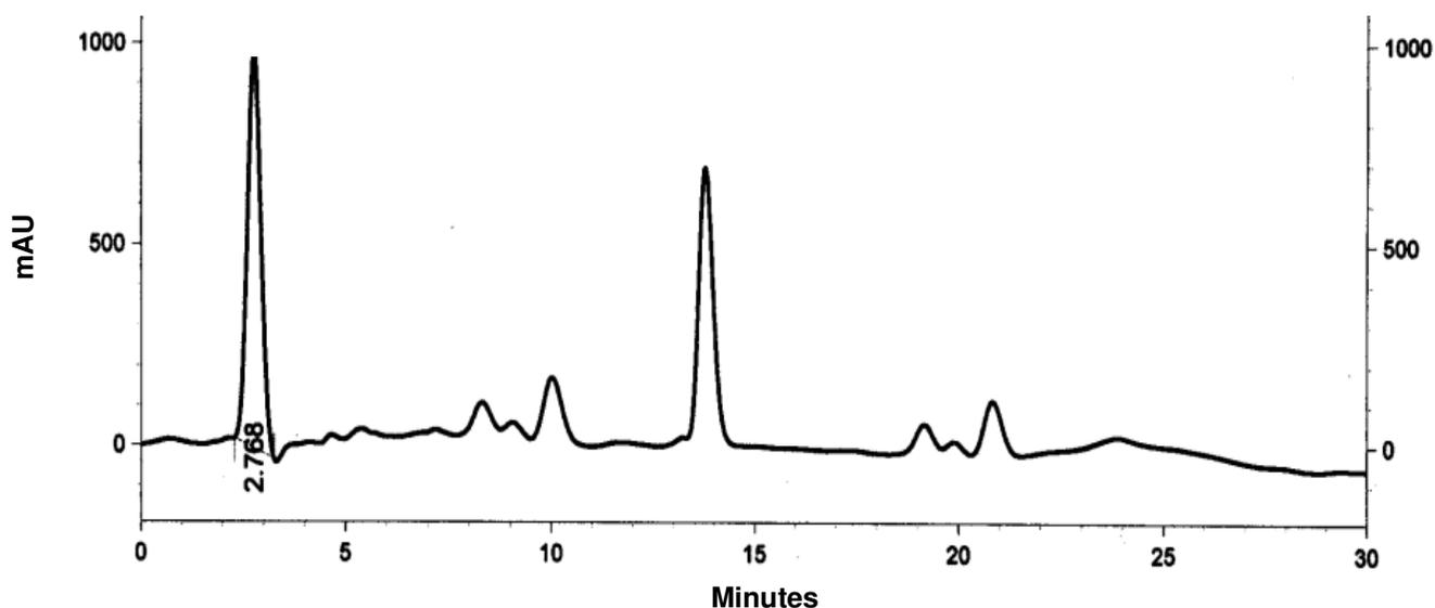
**Figure 1.** HPLC chromatogram of Sandimmun Neoral<sup>®</sup> capsule extracted at 215 nm. Peak at 2.7 is of Cyclosporin 'A'.
