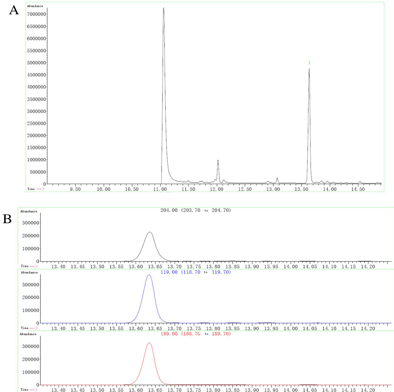
**Figure 1.** GC-MS identification of amorpho-4,11-diene produced by W303A[ADS]. A, The total ion chromatogram of W303A[ADS]; B, selected ion monitoring of W303A[ADS]; C, MS spectrum of the peak of retention time, 13.635 min.
