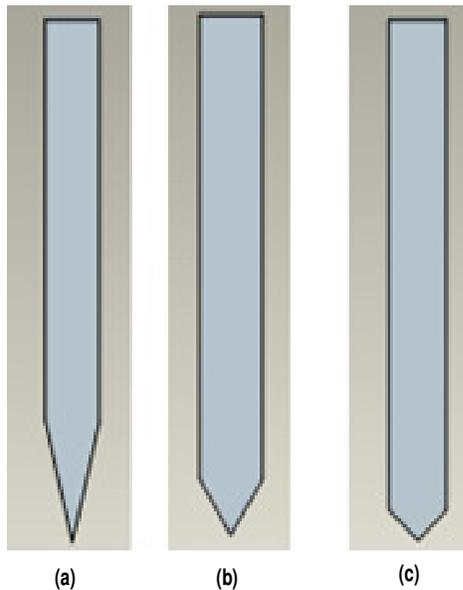
Figure 11. Testing cutters (a)  $\beta=30^\circ$ , (b)  $\beta=60^\circ$  and (c)  $\beta=90^\circ$ .
