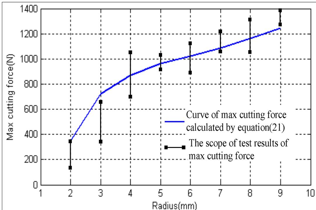
Figure 13. Max cutting force( $\beta=30^\circ$ ).
