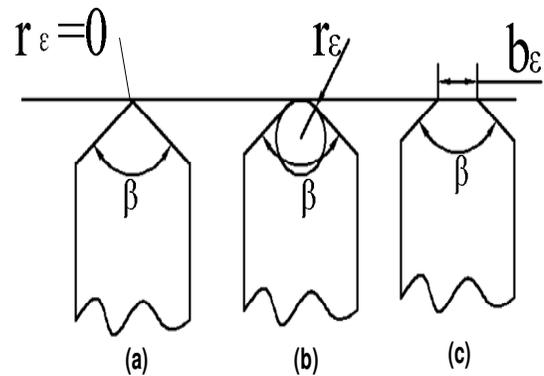
**Figure 3.** The shape of cut edge
