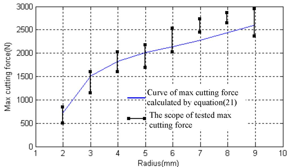
Figure 15. Max cutting force( $\beta = 90^\circ$ ).
