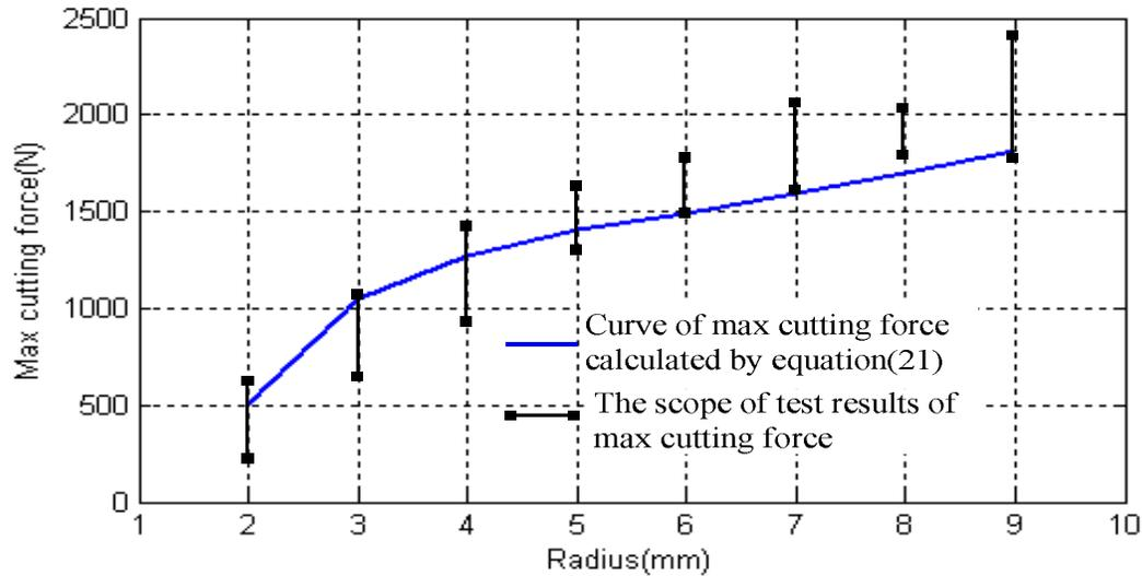
Figure 14. Max cutting force( $\beta= 60^\circ$ ).
