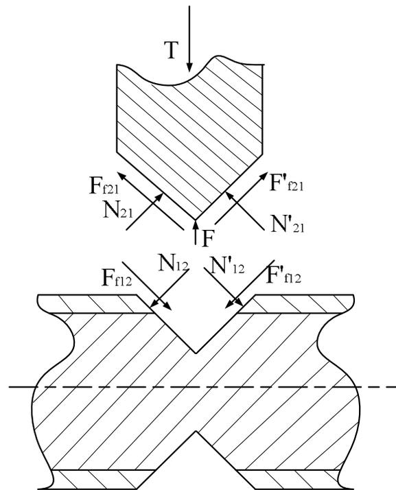
**Figure 4.** Interaction model between stalk and cutter.
