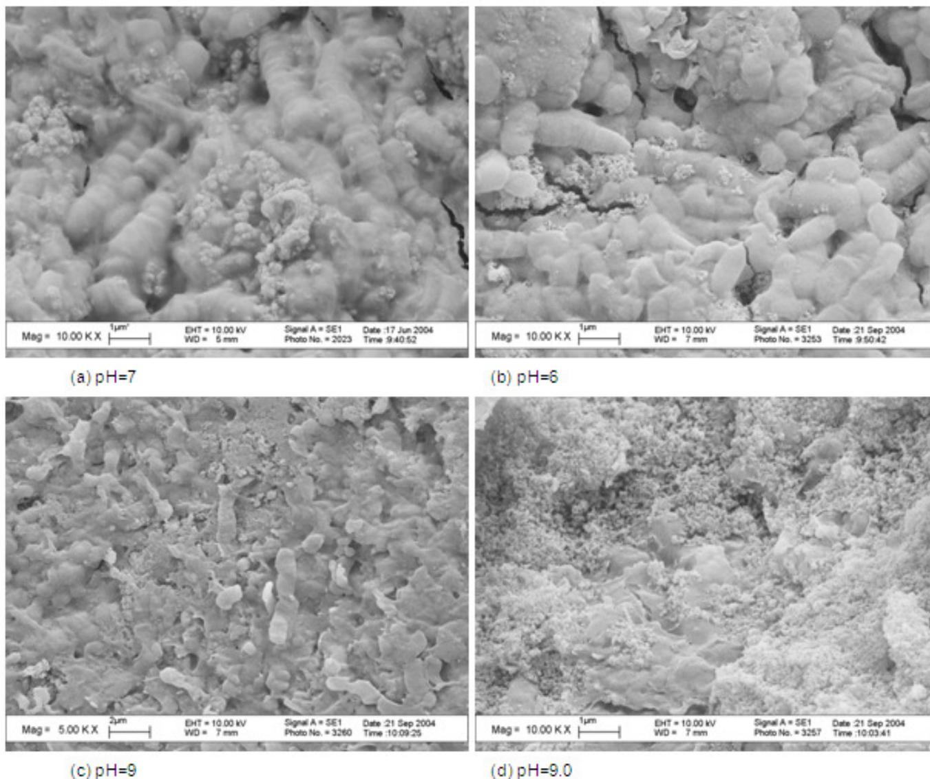
**Figure 5.** The microbial morphology of bacteria at different pH value.
