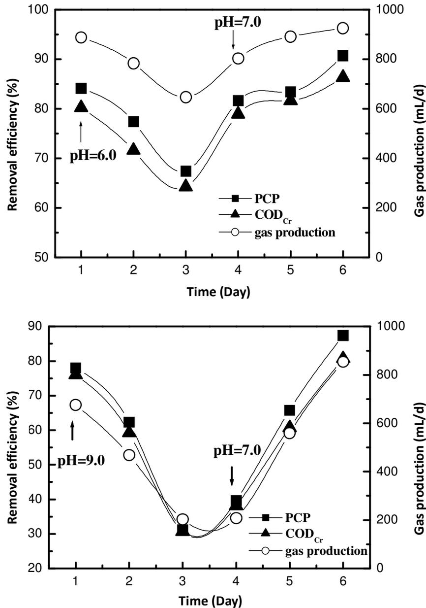
Figure 1. Effect of short time pH shock on reactor operation.
