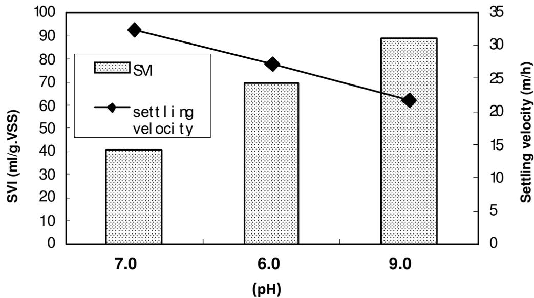
Figure 4. Effect of pH shock on SVI and settling velocity of the granular sludge
