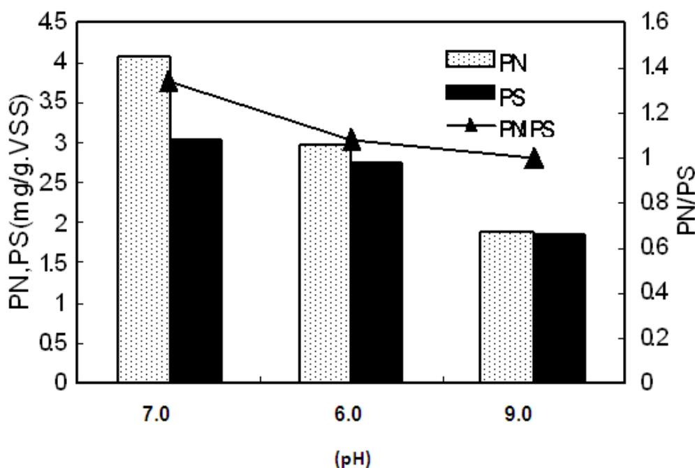
Figure 3. Effect of pH shock on extracellular polymers
