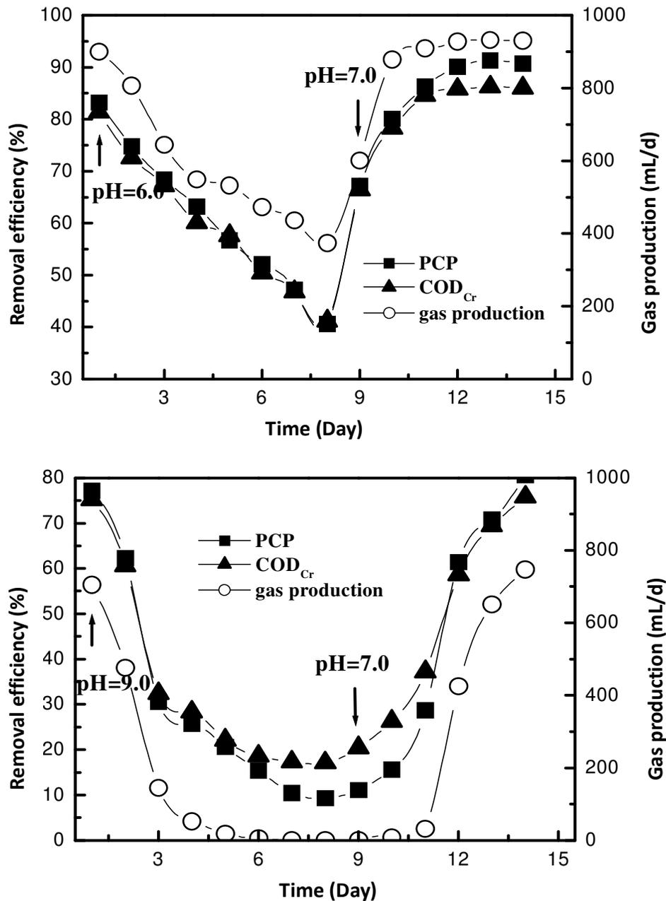
Figure 2. Effect of long time pH shock on the reactor operation.
