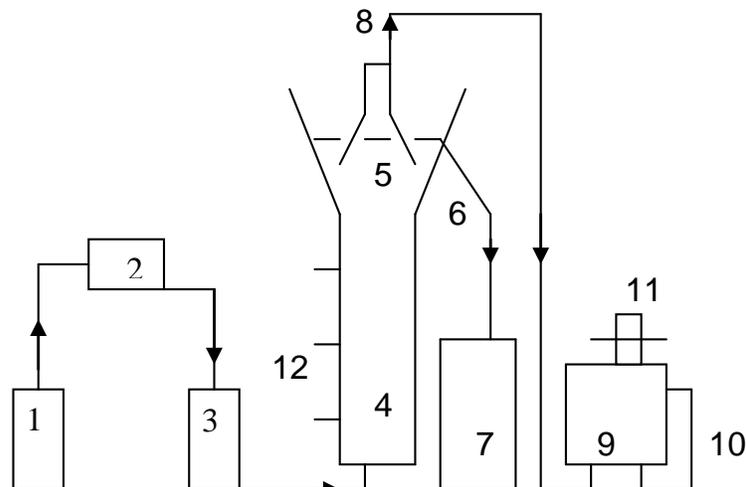
**Figure 1.** Schematic diagram for experimental set-up of the UASB reactor. 1, Waste water reservoir; 2, feeding pump; 3, heat exchange unit; 4, UASB reactor; 5, three-phase separator; 6, effluent overflow; 7, effluent collector; 8, gas outlet; 9, gas collector; 10, side-arm measuring device; 11, gas discharge valve; 12, sampling ports.
