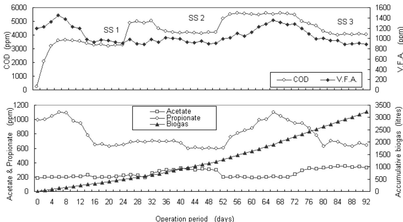
**Figure 3.** Performance of UASB reactor during continuous operation using industrial wastewater with different organic loading rates. SS1, steady state at 4 g COD/L/d; SS 2, steady state at 6 g COD/L/d ; SS 3, steady state at 8 g COD/L/d. COD values taken after excluding COD consumed in VFA synthesis.
