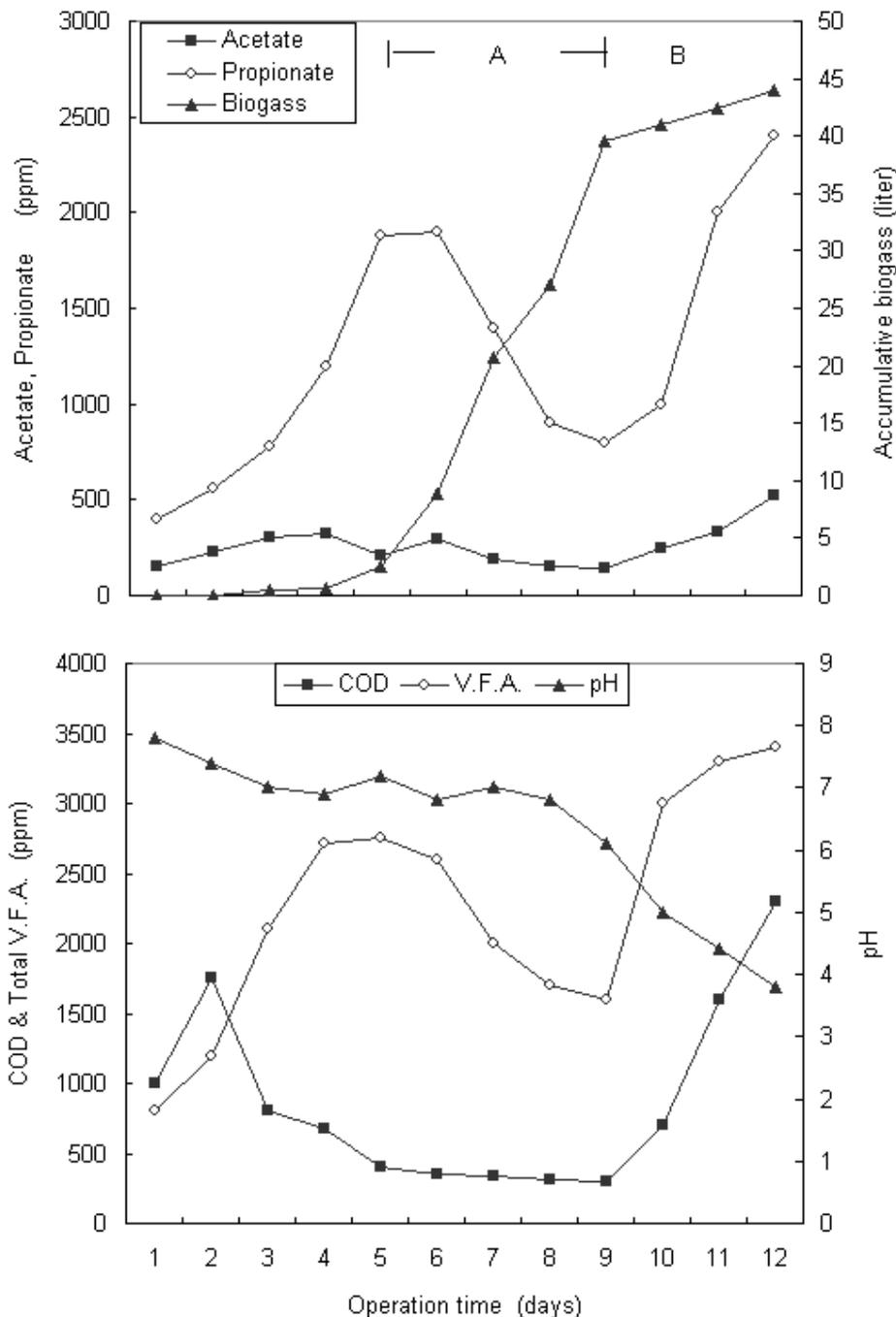
**Figure 2.** Performance of UASB reactor during fed-batch operation. A and B are operation stages between days 5, 9 and 12, respectively. COD value taken after excluding the amount of COD consumed in VFAs synthesis.
