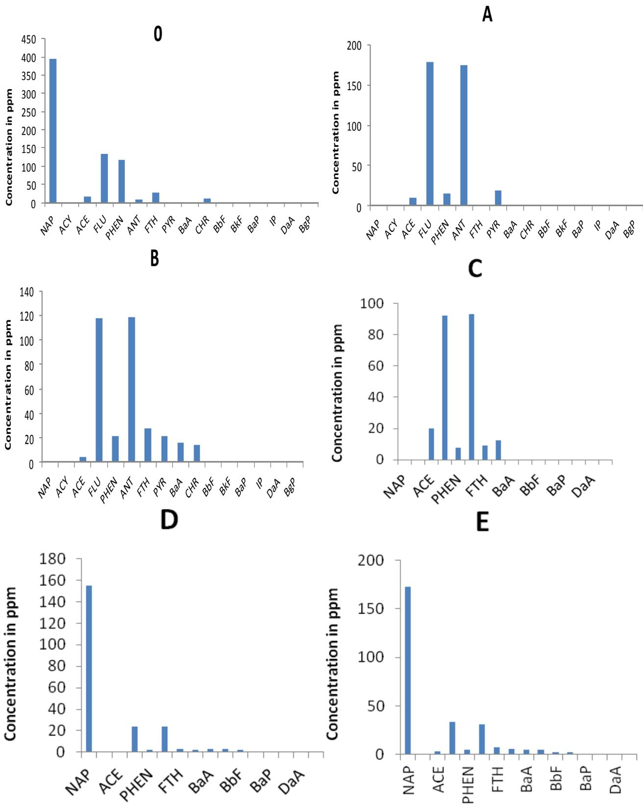
**Figure 3.** Polycyclic Aromatic Hydrocarbon (PAH) Profile of Biodegraded PFB. O = control,A = ANB sample degraded by *Pseudomonas putrefaciens*,B = ANB sample degraded by *Pseudomonas nigrificans*,C = ANB sample degraded by *Bacillus licheniformis*,D = ANB sample degraded by *Pseudomonas fragi*,E = ANB sample degraded by *Achromobacter aerogenes*
