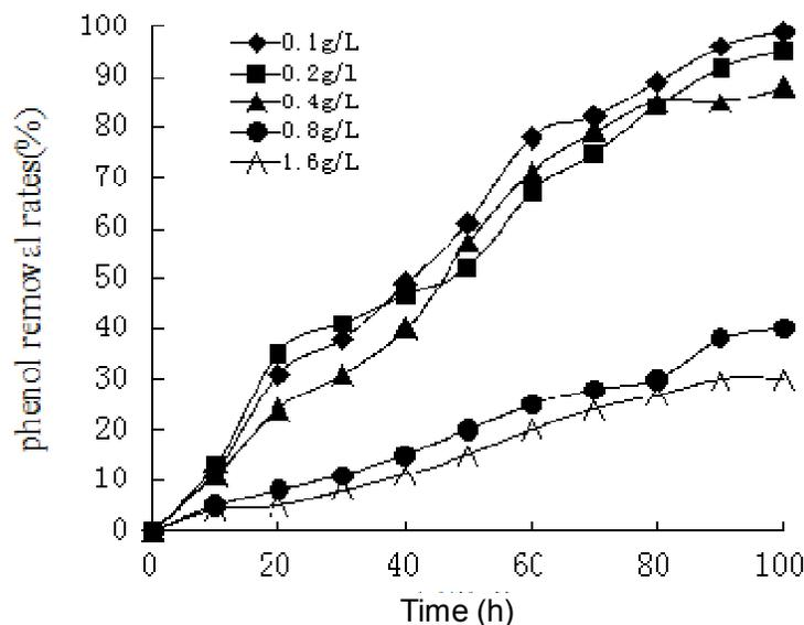
**Figure 1.** Phenol removal rates of strain SKDP-1 with phenol concentrations of 0.1, 0.2, 0.4, 0.8, 1.6 g/L in MSM medium at 100 h incubation, respectively.
