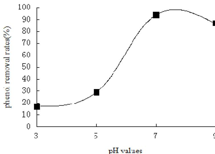
**Figure 2.** Phenol removal rates of strain SKDP-1 at 100 h incubation in MSM medium with different pH of 3, 5, 7 and 9, respectively.
