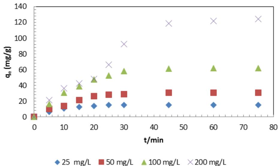
**Figure 7.** Effect of contact time on adsorption capacity of MB onto silica gel immobilized *Chlorophyta hydrodictyon africanum* for different initial dye concentrations (pH8, T=25°C, agitation speed =135 rpm, adsorbent dosage = 0.8 g·L<sup>-1</sup>).
