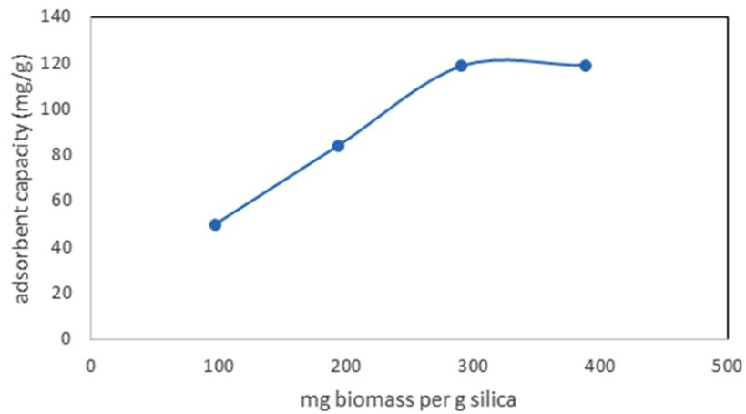
**Figure 5.** Effect of dosage level on maximum adsorption capacity of MB onto *Chlorophyta hydrodictyon africanum* encapsulated on to silica gel (pH8,  $t=90 \text{ min}$ ,  $T=25^\circ\text{C}$ , agitation speed = 135 rpm).
