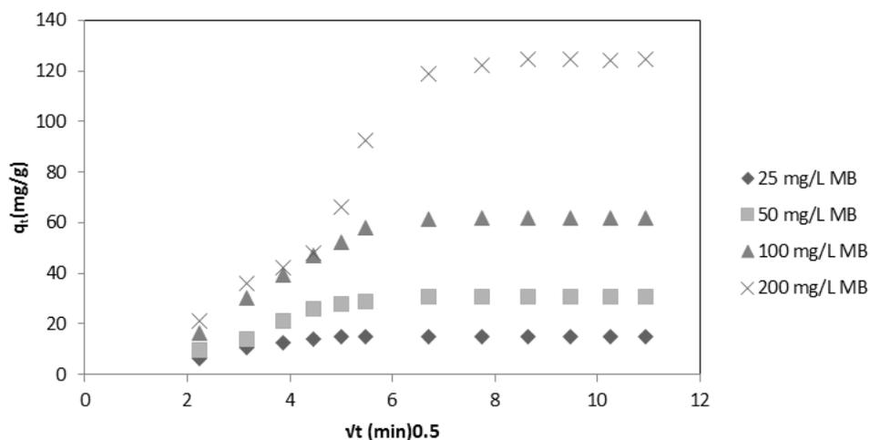
**Figure 10.** Intra-particle diffusion plot for the adsorption of MB using immobilized *Chlorophyta hydrodictyon africanum* (pH 8, adsorbent dosage = 1.6 g·L<sup>-1</sup> at 25°C).**Table 3.** Intra-particle diffusion parameters for the adsorption of MB on *Chlorophyta hydrodictyon africanum* immobilized of silica gel.
