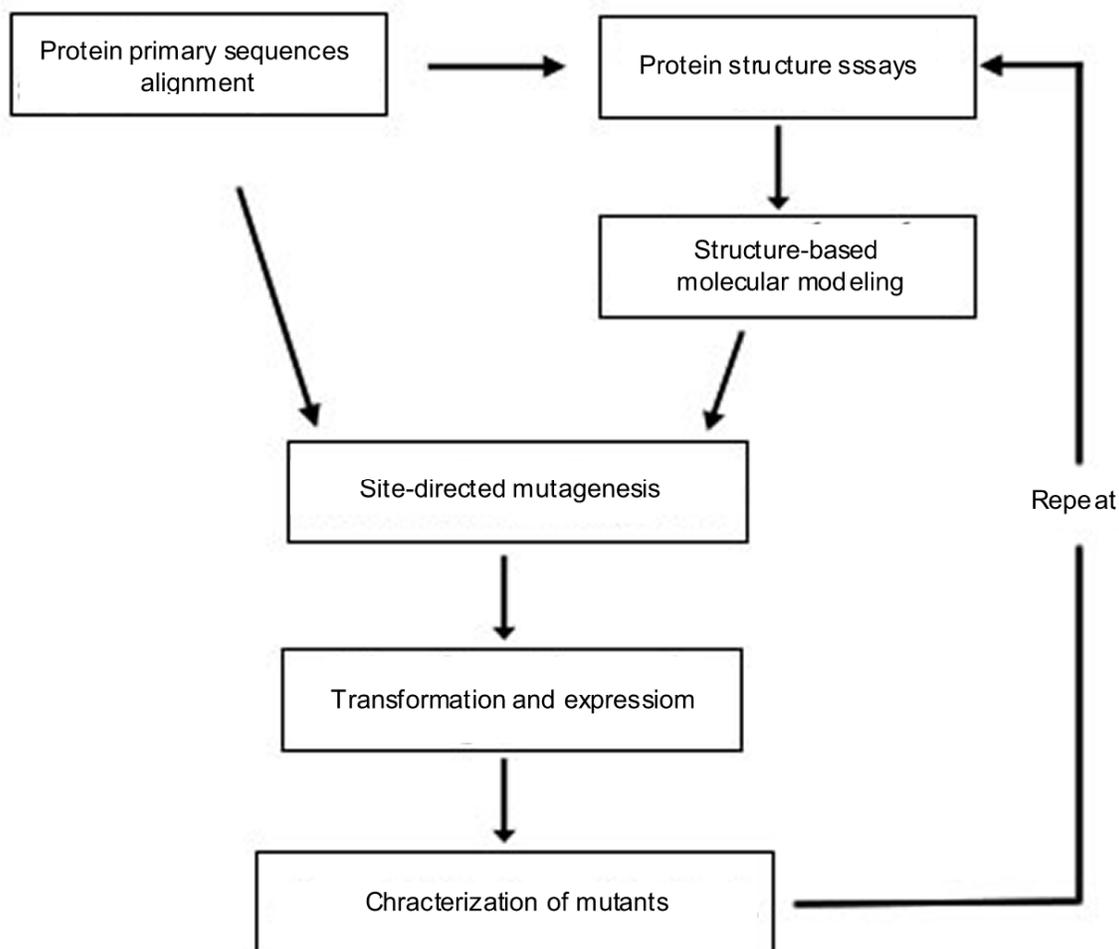
**Figure 4.** Schematic diagram of rational design. Protein primary sequences alignment and structure-based molecular modeling are usual foundation of rational protein design, and then site-directed mutagenesis is performed to prove the hypotheses. The whole process is often repeated until the improved gene(s) obtained.
