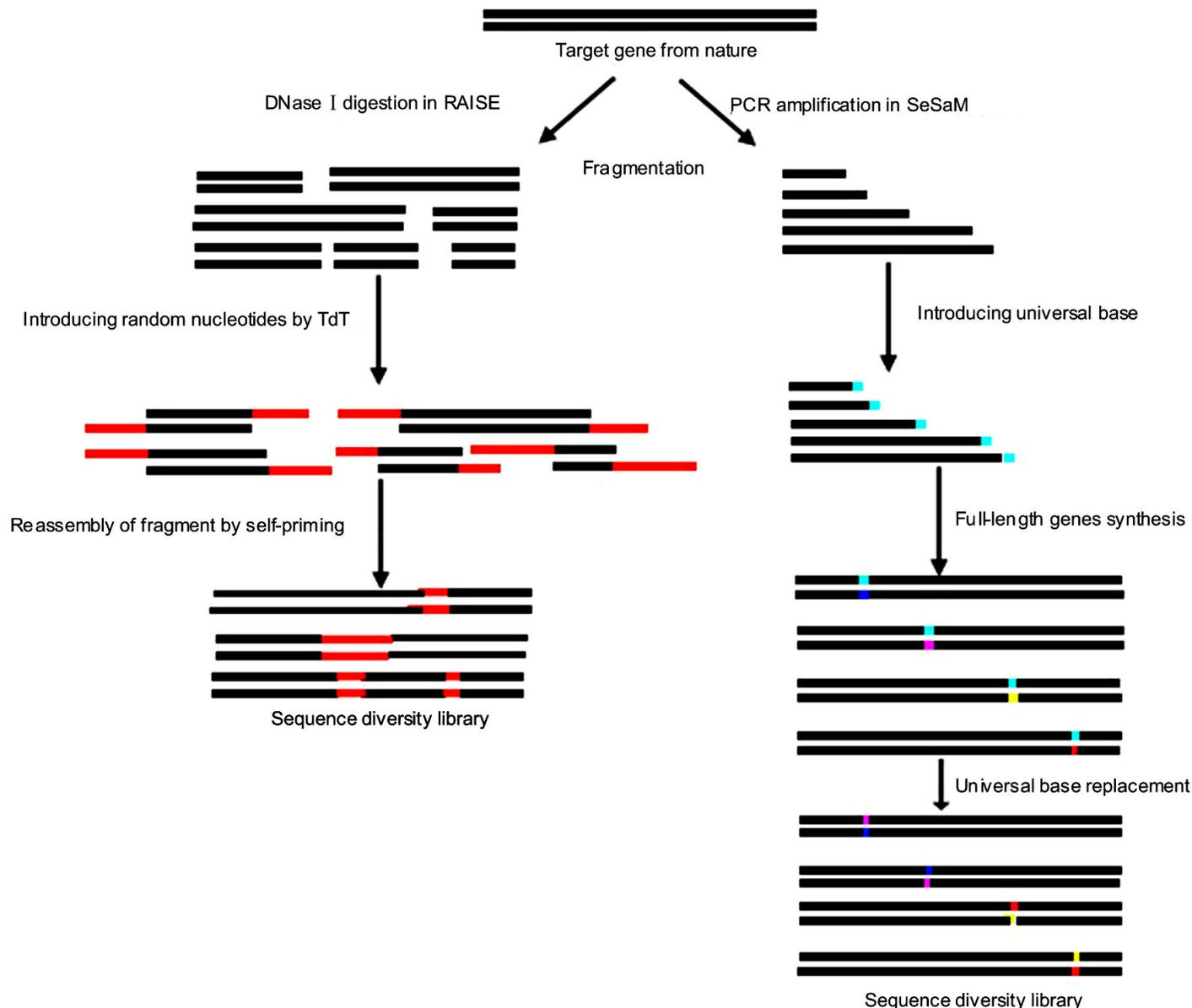
**Figure 3.** Schematic diagram of RAISE and SeSaM. RAISE and SeSaM are both starting at DNA fragmentation. In RAISE, the fragments are attached with random nucleotides by TdT, and then reassembled by self-priming. In SeSaM the fragments are introduced universally base by terminal transferase at 3' terminus, followed by full-length synthesis and universal base replacement with standard bases, which are labeled with different color in the figure.
