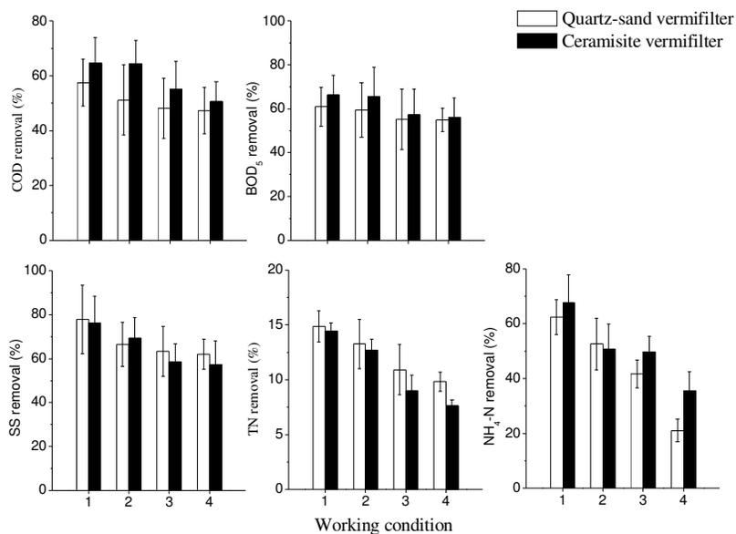
**Figure 2.** Removal rates of wastewater in four working conditions of both vermicilters. Values are means, bars are S.E., and  $n = 4$ .
