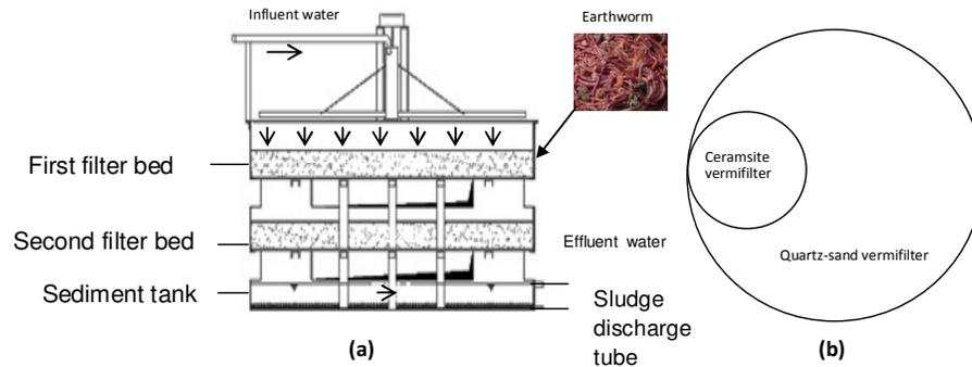
**Figure 1.** Schematic diagram of vermifilter. a) front view; b) top view (Ceramsite vermifilter was included in quartz-sand one).
