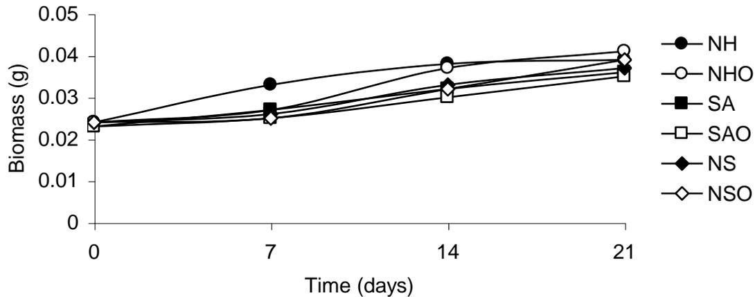
**Figure 2.** Biomass quantified by dry weight analysis during bioremediation; NH, *N. hatei*; NHO, *N. hatei* in used motor oil; SA, *S. aquatilis*; SAO, *S. aquatilis* in used motor oil; NS, *N. hatei* + *S. aquatilis*; NSO, *N. hatei* + *S. aquatilis* in used motor oil.
