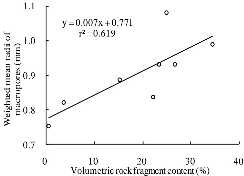
**Figure 4.** Influence of volumetric content of rock fragments on weighted mean radii of macropores in 8 plots.
