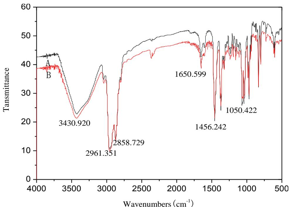
**Figure 3.** Infrared spectrogram of ergosterol crystal. The infrared spectrum was obtained on the infrared furrier spectrometer with KBr pellets in the region of 4000-400  $\text{cm}^{-1}$ . FTIR,  $\bar{\nu}$  ( $\text{cm}^{-1}$ ): 3430.920, 2961.351, 2858.729 and 1650.599. A, Standard sample of ergosterol; B, the ergosterol produced by corn straw.
