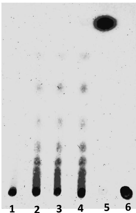
**Figure 7.** TLC of hydrolysis products of birchwood xylan upon reaction with a purified extracellular xylanase from *A. terreus*. Lanes 1 to 4, hydrolysis products using xylanase I after 0, 30, 60 and 420 min of incubation, respectively; lanes 5 and 6, hydrolysis products of the standards (xylose and xylan, respectively).
