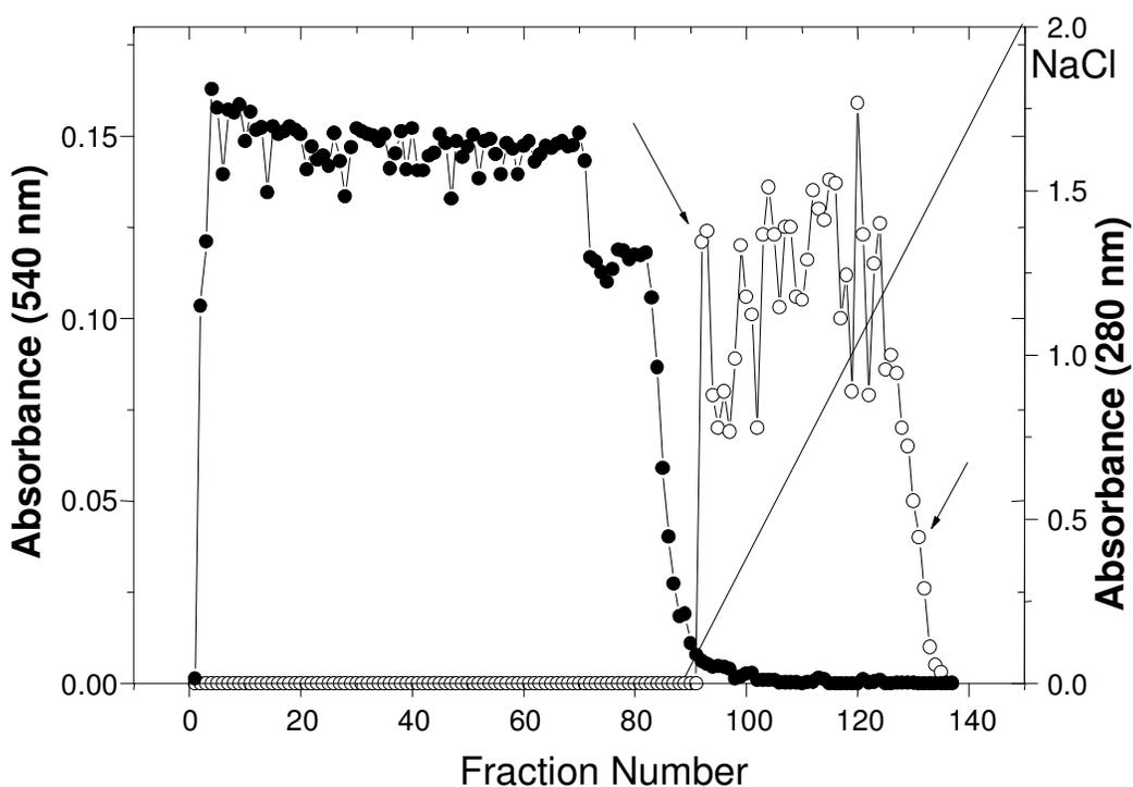
**Figure 2.** CM-cellulose ion exchange chromatography of a xylanase produced by *A. terreus*. Arrows indicate pooled fractions exhibiting xylanase activity. The column was equilibrated with 50 mM acetate buffer at pH 4.5 and eluted with a linear salt gradient (0 to 1 M) in the same buffer. Flow rate and fraction size were 50 ml/h and 5.0 ml, respectively. ●, A280; ○ xylanase activity; —, NaCl concentration.
