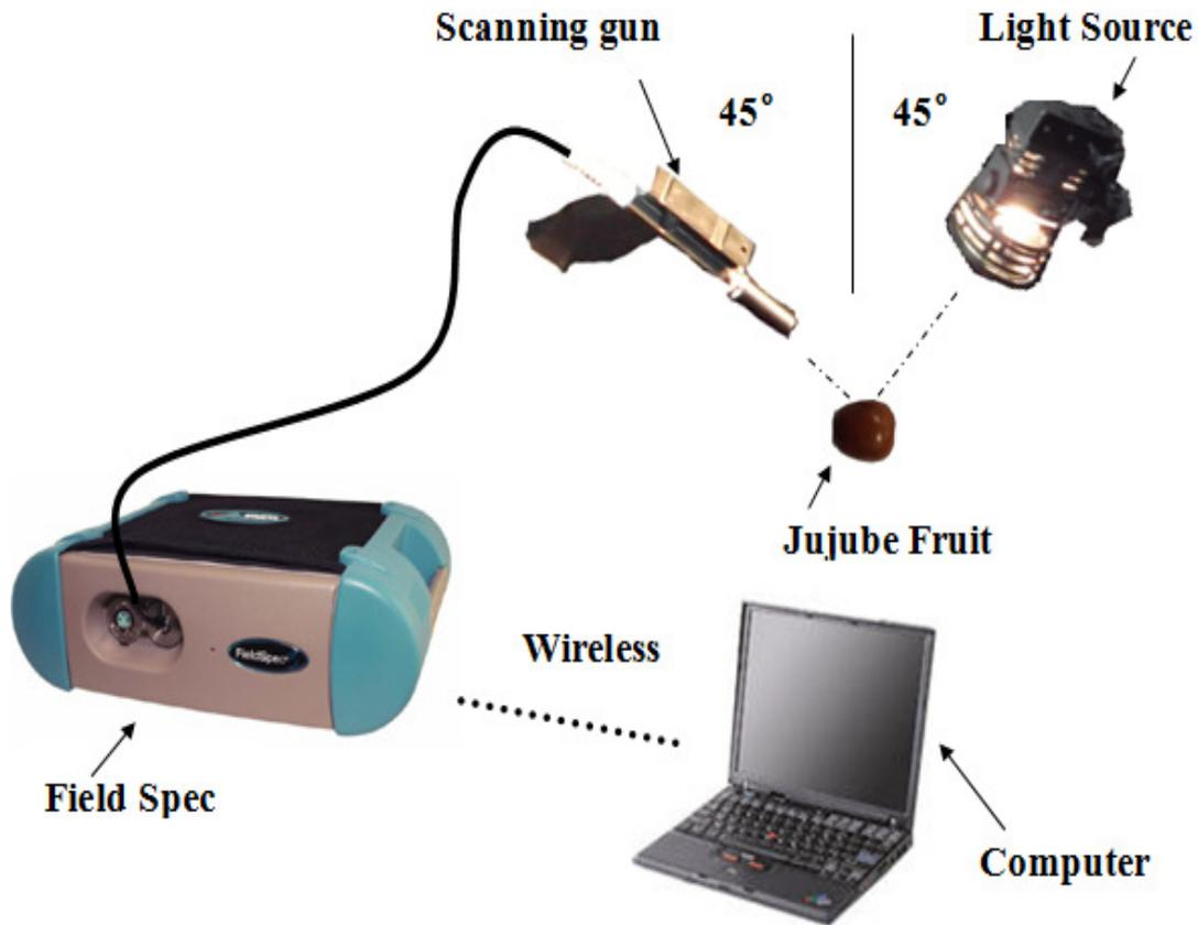
Figure 1. Visible near-infrared measurement equipment.
