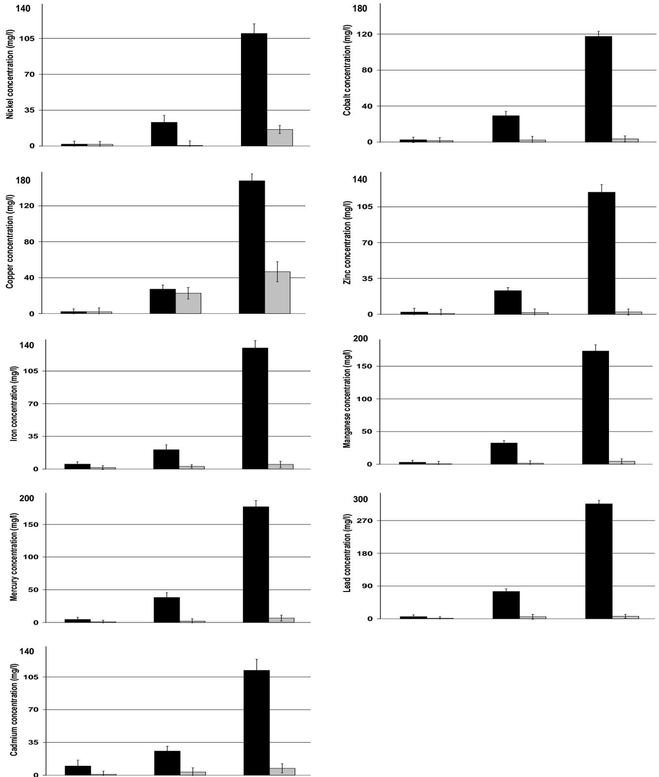
**Figure 3.** Metal bioprecipitation using the biogas produced from an aerobic bacterial culture of the activated sludge against different concentrations of metals as single metal species after 24 h of exposure time. Black columns indicate the initial concentrations while the grey columns indicate the final concentrations. Data are the means of three replicates. Error bars represent the standard errors of the means.
