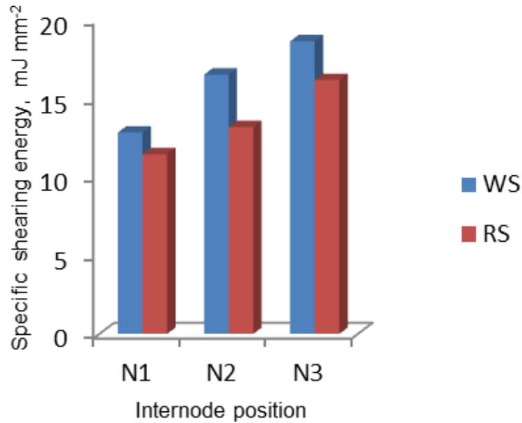
**Figure 8.** Influence of specific shearing energy of WS and RS at different internode position under 20 mm min<sup>-1</sup>.
