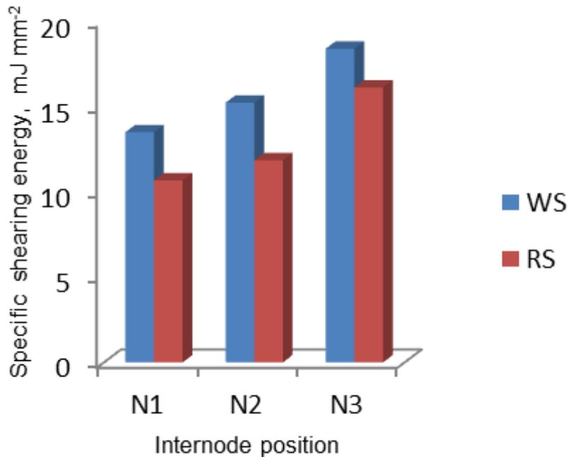
**Figure 9.** Influence of specific shearing energy of WS and RS at different internode position under 25 mm min<sup>-1</sup>.
