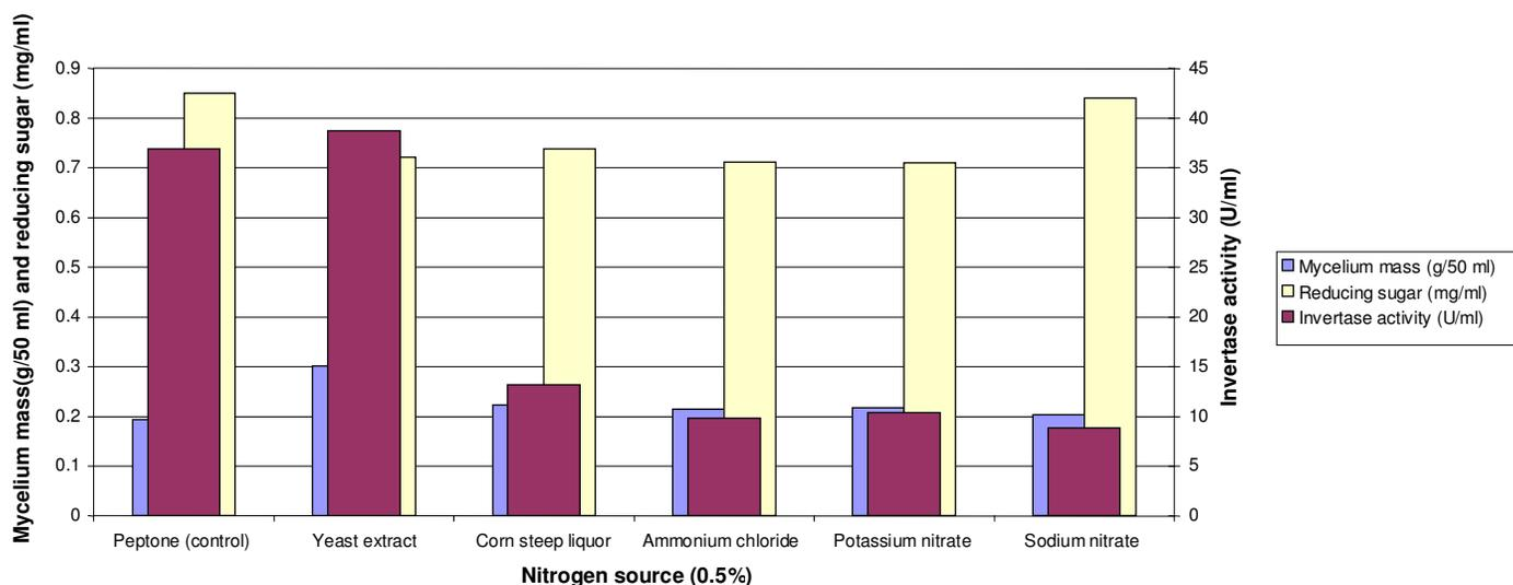
**Figure 5.** Effect of nitrogen source (5 g/l initial concentration) on invertase production, biomass concentration and residual reducing sugar level at 48 h of fermentation (30°C, initial pH of 6.5) in a *Brassica niger* (10 g/l initial concentration) mineral medium.
