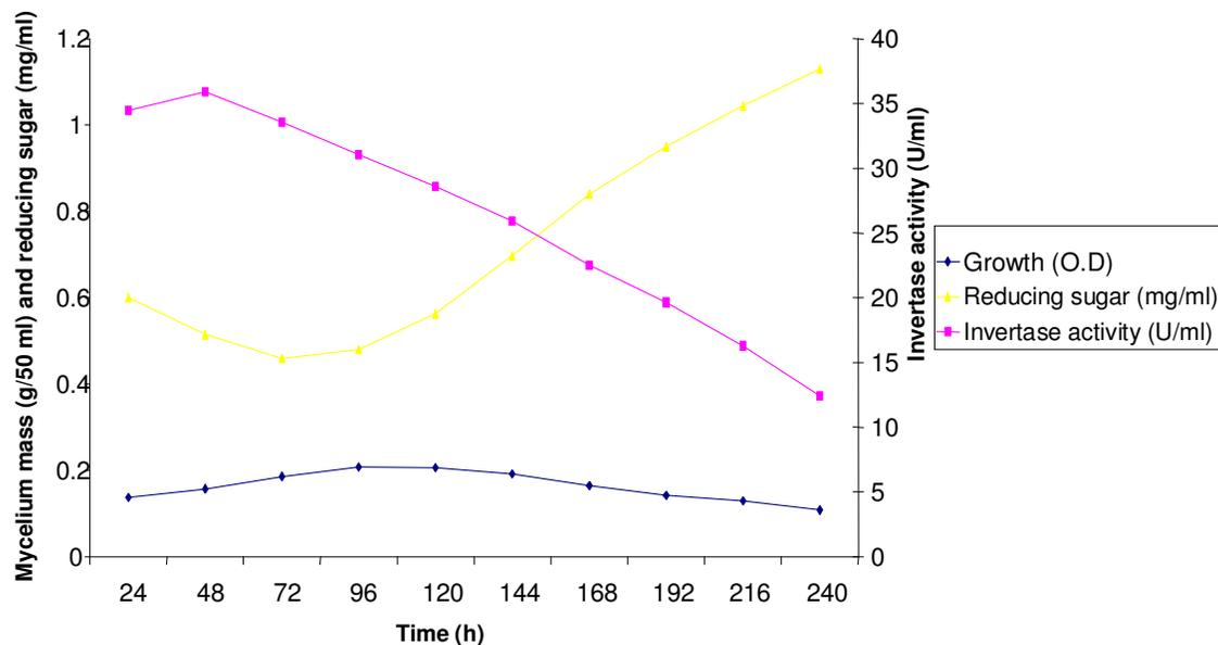
**Figure 1.** Batch profiles of biomass growth, invertase activity and reducing sugar concentration during enzyme production (30°C, initial pH of 6.5).
