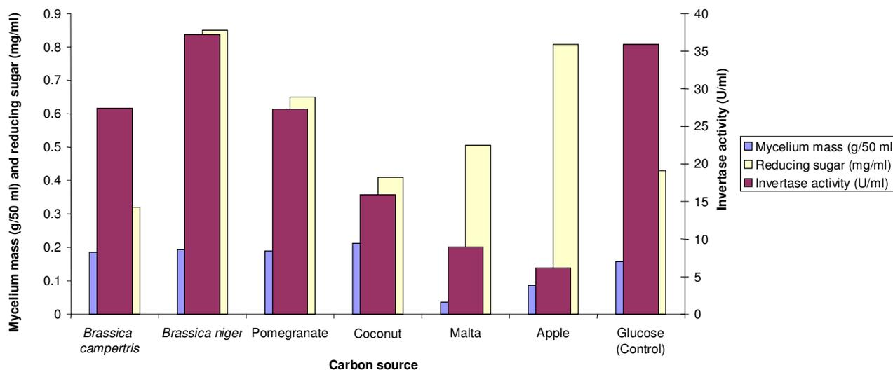
**Figure 2.** Effect of fruit waste and oil cake as carbon source (10 g/l initial concentration) hydrolyzed with 0.3 N HCl on biomass concentration, invertase activity and residual reducing sugar level at 48 h of fermentation (30°C, initial pH of 6.5).
