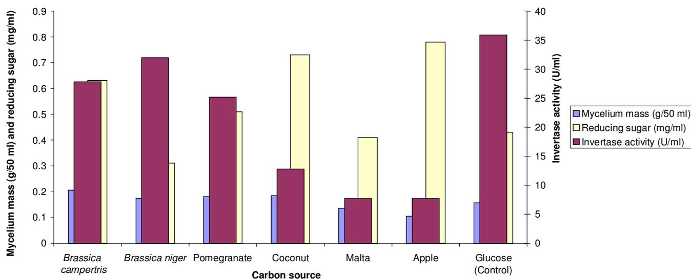
**Figure 3.** Effect of fruit waste and oil cake as carbon source (10 g/l initial concentration) hydrolyzed with 0.6 N HCl on biomass concentration, invertase activity and residual reducing sugar level at 48 h of fermentation (30°C, initial pH of 6.5).
