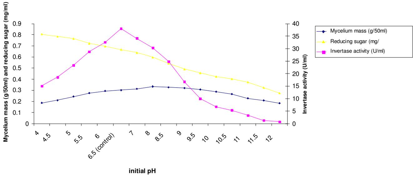
**Figure 6.** Effect of initial pH on invertase production, biomass growth and residual sugar concentration at 48 h of fermentation (30°C) in a mineral medium containing *Brassica niger* hydrolyzed with 0.3 N HCl and yeast extract at initial concentrations of 10 and 5 g/l, respectively.
