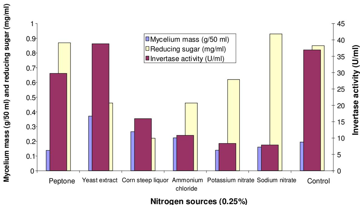
**Figure 4.** Effect of nitrogen source (2.5 g/l initial concentration) on invertase production, biomass concentration and residual reducing sugar level at 48 h of fermentation (30°C, initial pH of 6.5) in a *Brassica niger* (10 g/l initial concentration) mineral medium.
