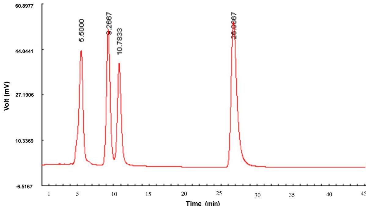
**Figure 3.** HPLC Diagram of mixture of nucleoside standard sample (i) uridine (ii) inosine (iii) guanosine (iv) adenosine.
