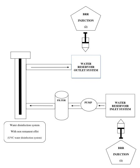
Figure 4. Application of bio-remanent reagent (BRR) injection process inlet (1) or/and outlet (2) disinfection system.
