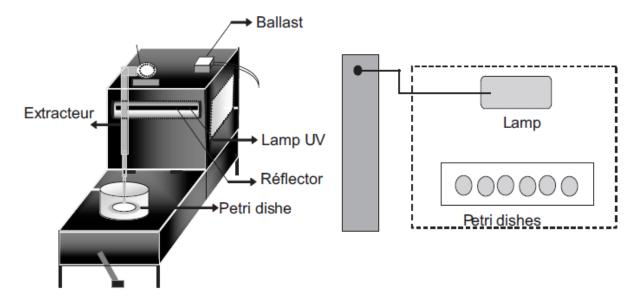
Figure 1. Experimental setup for UVC irradiation.
