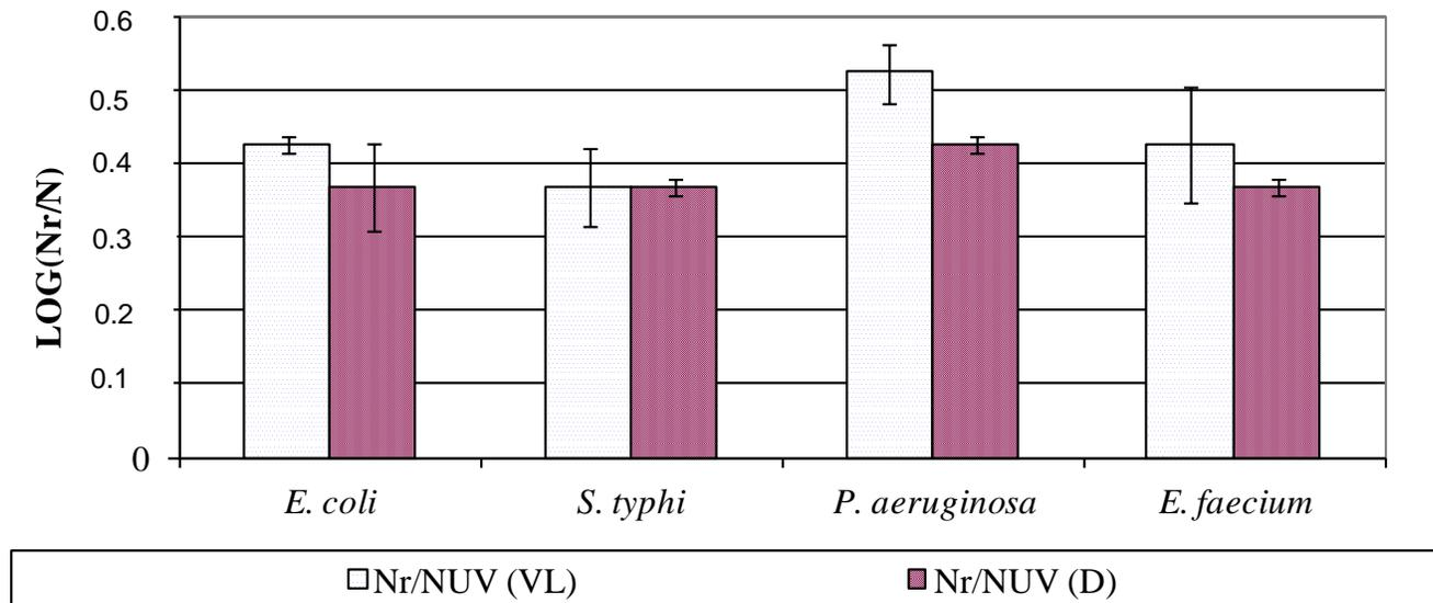
**Figure 3.** Bacterial reactivation ( $C_R$ ) or log increase in the presence of photoreactivation and dark repair conditions after UVC irradiation with addition of biological remanent reagent (BRR).  $N_{UV}$  is the number of viable and cultivable bacteria after UVC irradiation;  $N_{VL}$  and  $N_D$  are the number of recovered bacteria after a rest time in the presence of visible light (VL) and in darkness (D).
