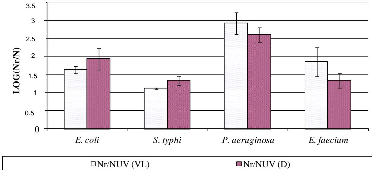
**Figure 2.** Coefficient of bacterial reactivation ( $C_R$ ) or log increase in the presence of photoreactivation and dark repair conditions after UVC treatment without addition of biological remanent reagent (BRR).  $N_{UV}$  is the number of viable and cultivable bacteria after UVC irradiation;  $N_{VL}$  and  $N_D$  are the number of recovered bacteria after a rest time in the presence of visible light (VL) and in darkness (D).
