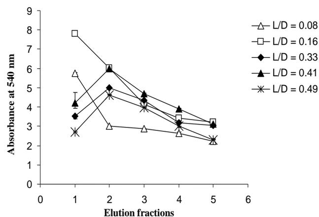
**Figure 7.** Absorbance readings of 5 elution fractions obtained from varying adsorbent height (L) in a column having a constant internal diameter (D) of 2.45 cm. Translating the absorbance readings of  $\alpha$ -amylase concentration in the various purified elution fractions into activities, the highest activity was 75.549 U/ml.
