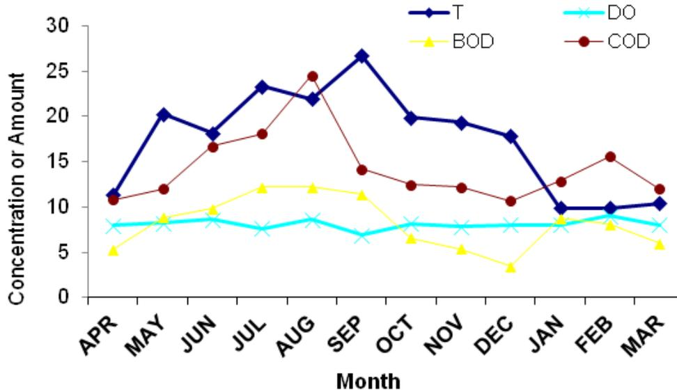
**Figure 5.** The trend of mean concentration variations of Temperature (°C), BOD (mg/l), DO (mg/l) and COD (mg/l) in Tajan River in different stations.
