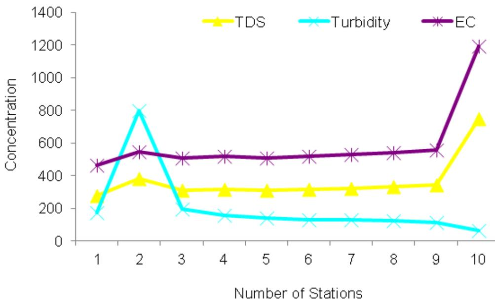
**Figure 2.** The trend of concentration variations of turbidity (NTU), electrical conductivity ( $\mu\text{s}/\text{cm}$ ) and total dissolved solids (mg/l) in Tajan River at 10 sampling stations.
