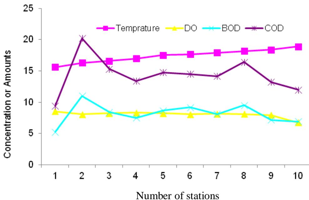
**Figure 3.** The trend of concentration variations of temperature ( $^{\circ}\text{C}$ ), BOD (mg/l), DO (mg/l) and COD (mg/l) in Tajan River at 10 sampling stations.
