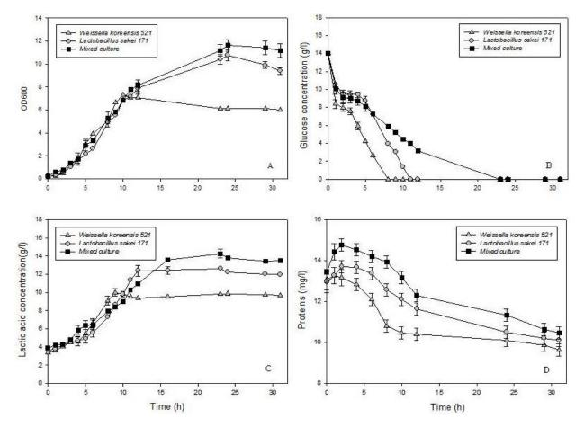
**Figure 2.** Changes of growth, glucose contents, lactic acid produced and total protein used during fermentation by single and mixed cultures of kimchi lactic acid bacteria. Each number represents the mean  $\pm$  SD of three replicates.
