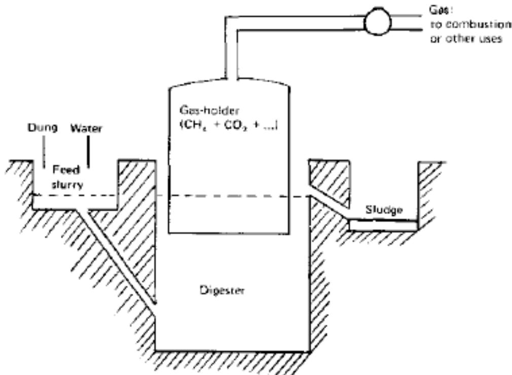
Figure 3. Floating-drum plant.
