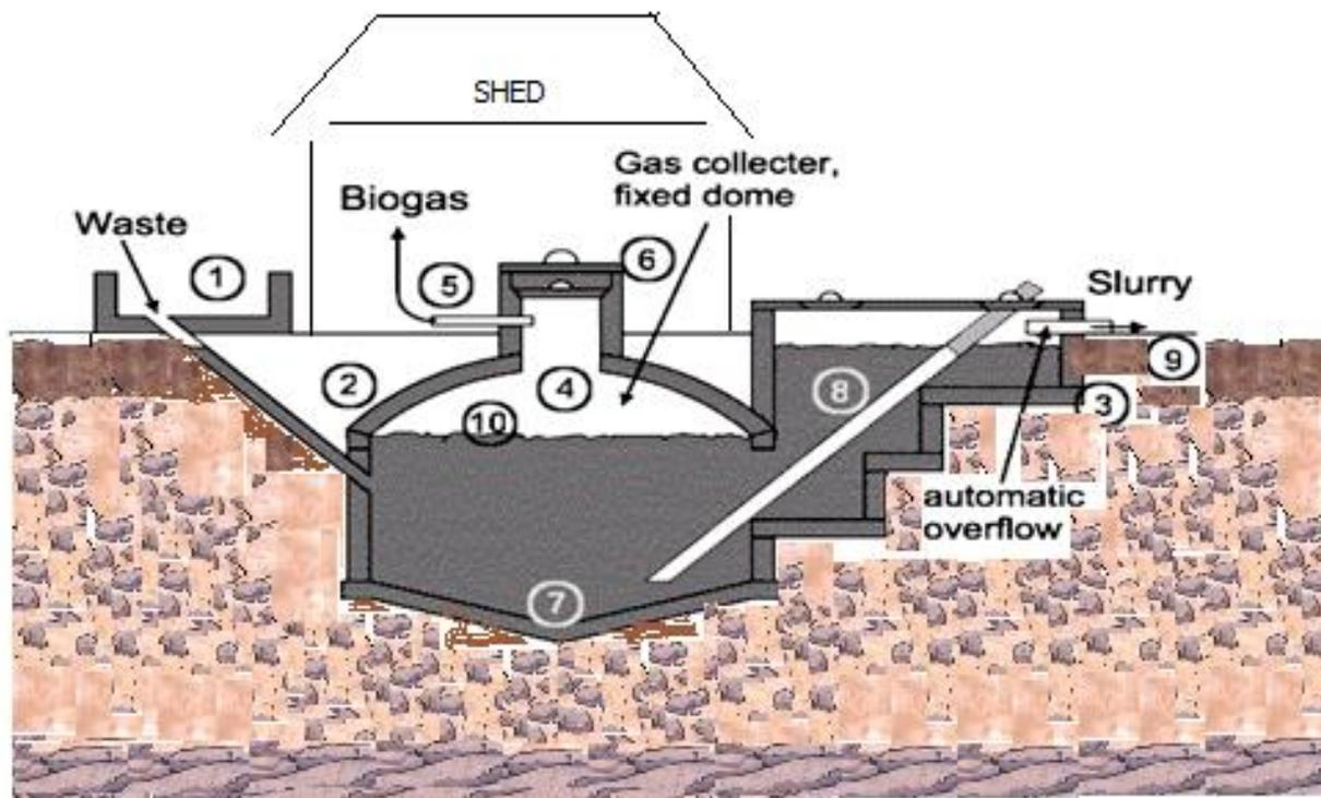
**Figure 2.** Fixed dome plant Nicarao design. 1. Mixing tank with inlet pipe and sand trap. 2. Digester. 3. compensation and removal tank. 4. Gas holder. 5. Gas pipe. 6. Entry hatch, with gastight seal. 7. Accumulation of thick sludge. 8. Outlet pipe. 9. Reference level. 10. Supernatant scum, broken up by varying level (GTZ, 1999).
