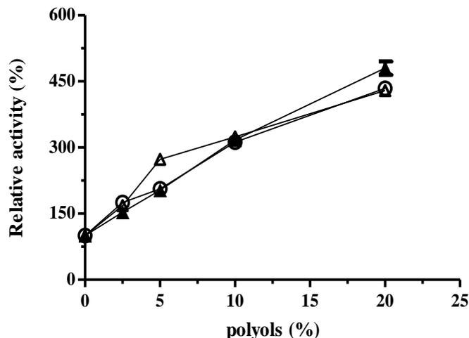
**Figure 4.** Thermostability of the xylanase at 50°C, with manitol (▲), xylitol (●) and glycerol (Δ) in different concentrations [2.5 – 20% (w/v)]. Residual activity was assayed after 120 min at 50°C.
