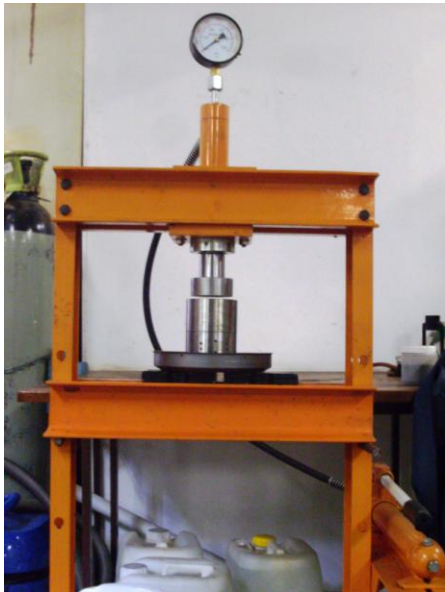
Figure 1. Custom-built hydraulic cold press.
