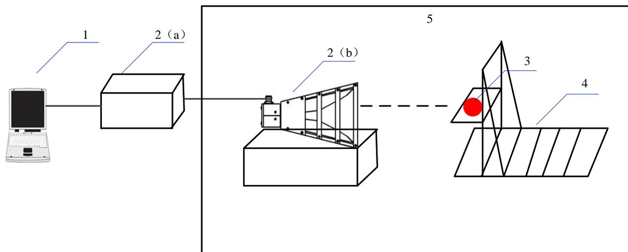
**Figure 1.** Schematic diagram of the irradiation platform. 1, Computer; 2, microwave irradiator; 2(a), microwave source; 2(b), antenna; 3, animal; 4, 2D objective table; 5, microwave anechoic chamber.
