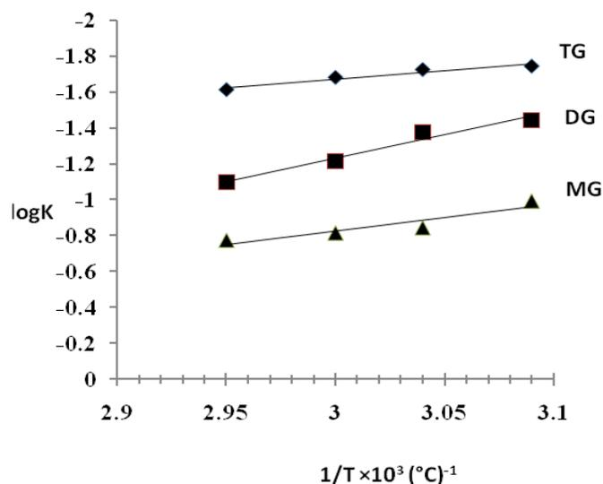
**Figure 6.** Arrhenius plot of reaction rate with reciprocal temperature.
