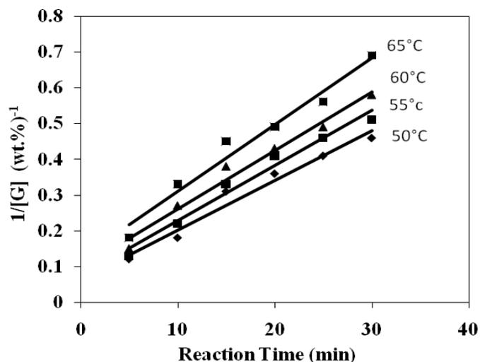
**Figure 5.** Rate constant plot for glycerides at different temperatures.
