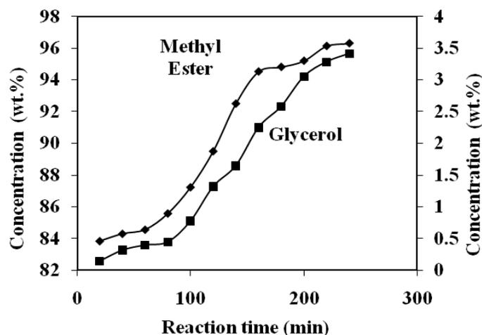
Figure 2. Biodiesel and glycerol conversion with reaction time.
